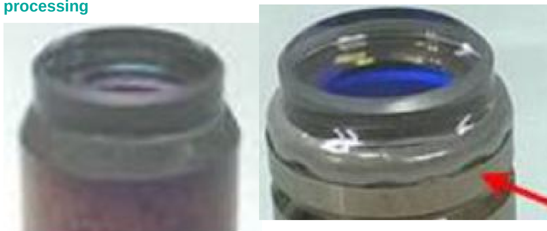
Figure 32-2: Lead-based (left) and bismuth-based frit (right) after processing
