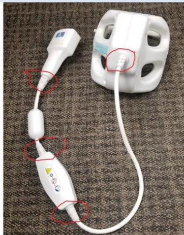
Figure 7-1: MRI coil for shoulder; the four strain relief boots are circled in red.
